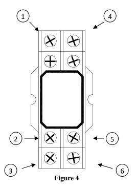
For section A of this relay, the terminal identified as item 1 in figure 4 is the Common contact, the terminal identified as item 2 is the Normally Closed (NC) contact and the terminal identified as item 3 is the Normally Open (NO) contact.
