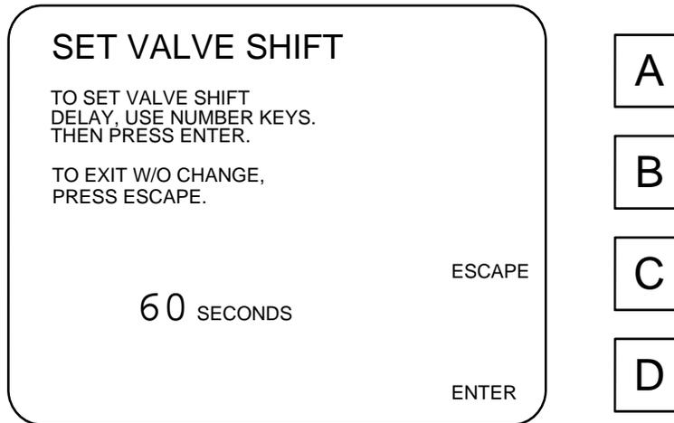
**Figure 2,** Set Valve Shift
